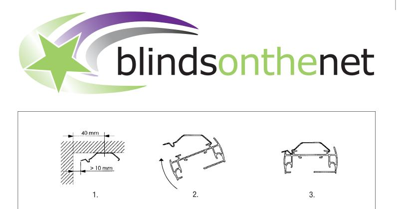
Install brackets ensuring there is a small clearance behind the headrail for the constant pleat clips on back of blind
